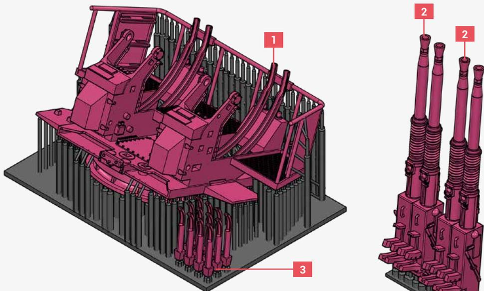
TO FREE PART 1, IT IS RECOMMENDED TO FIRST REMOVE THE OUTER SUPPORTS USING EITHER A SHARP BLADE OR MICRO-SAW, THEN SANDING OR SMOOTHING DOWN ANY REMAINING TABS FROM THE RAILINGS. AFTERWARDS REMOVE THE REMAINING SUPPORTS WORKING FROM THE OUTSIDE INWARD.
